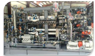
Offshore Ultrapure Water Generation Package
