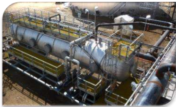
Onshore Deoiling Water Treatment
