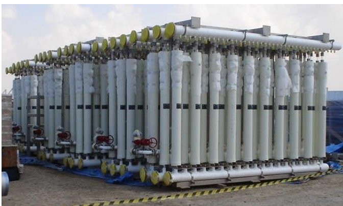
Photo: Offshore MF units (Courtesy of Pall Water)
